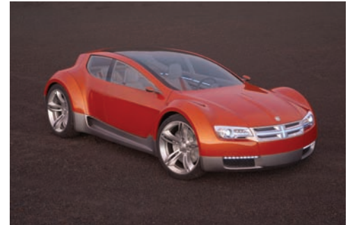
The roof of the Dodge Zeo concept is a continuous piece of laminated glass.
