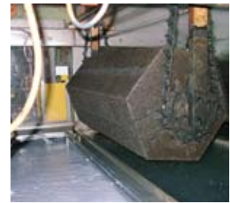
Figure 1: Barrel full of fasteners is transported from a black electrocoating tank to the rinse tank. Bulk electrocoat offers high-quality, high-throughput and lower overhead costs.
