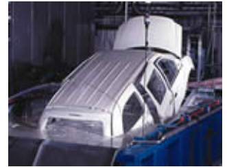
A car body emerges from one of the Flint facility's two 28,000 ft 2 e-coat tanks.
