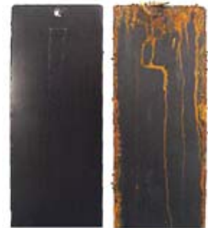
Figure VI: FrameCoat electrocoat vs. hot wax: 20 cycle Ford
