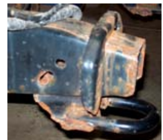
Figure V: FrameCoat electrocoat: 60 cycle Ford APG
