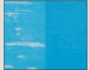
Example of leading competitor substrate with efflorescence (left). Substrate treated with Perma-Crete 4-2 primer (right).
